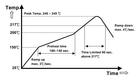
Recommended Temperature Profile for Lead-free Reflow Soldering Note: The temperature is measured on solder joint of pins of power module.
