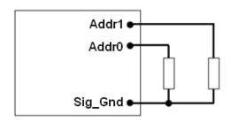
Corresponded to each octal digit, the requested resistor values are shown in below, and +/-1% resistors accuracy can be accepted. If there are any resistances exceeding the requested range, address 126 will be return. 0-12 and 40, 44, 45, and 55 in decimal address can't be used, since they are reserved according to the SMBus specifications, and which will also return address 126.
