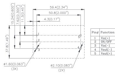
NOTES: DIMENSIONS ARE IN MILLIMETERS AND (INCHES) TOLERANCES: X.Xmm±0.5mm(X.XX in.±0.02 in.) X.XXmm±0.25mm(X.XXX in.±0.010 in.)
