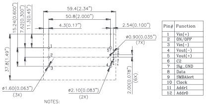
DIMENSIONS ARE IN MILLIMETERS AND (INCHES) TOLERANCES: X.Xmm±0.5mm(X.XX in.±0.02 in.)
