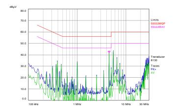
Figure 12-2: Test Result of EMC(Vin=54V, Io=60A).
