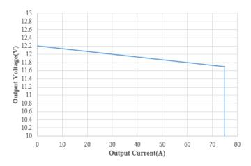
Figure 3: Output Voltage vs. Output Current showing typical current limit curves and converter shutdown points. Vin=54V
