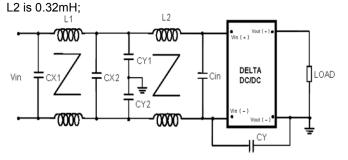
Figure 12-1: Recommended Input Filter
