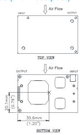
Figure 16: Hot spot 1 temperature measurement location The allowed maximum hot spot 1 temperature is defined at 120  $\mathcal{C}$ .
