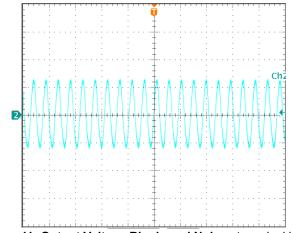
Figure 11: Output Voltage Ripple and Noise at nominal input voltage and max load current (20 mV/div, 2us/div) Load cap: 1100uF,(1000uF Oscon, 100uF ceramic).
