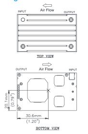
Figure 20: Hot spot 3 temperature measurement location The allowed maximum hot spot 3 temperature is defined at 120  $\mathcal{C}$ .
