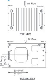
Figure 18: Hot spot 2 temperature measurement location The allowed maximum hot spot 2 temperature is defined at 120  $\mathcal{C}$ .
