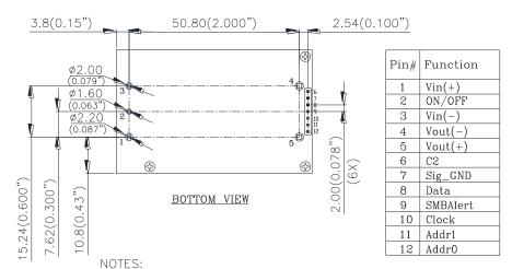
DIMENSIONS ARE IN MILLIMETERS AND (INCHES) TOLERANCES: X.Xmm±0.5mm(X.XX in.±0.02 in.) X.XXmm±0.25mm(X.XXX in.±0.010 in.)
