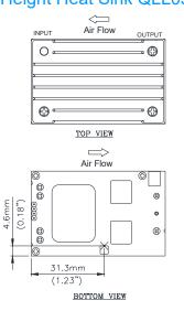
Figure 21: Hot spot 3 temperature measurement location
