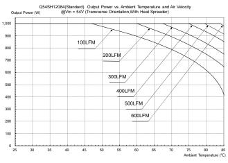
**Figure 18:** Output Power vs. Ambient Temperature and Air Velocity @Vin = 54V (Transverse Orientation, Airflow from Vin+ to Vin-, With Heat-spreader)
