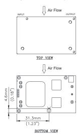
**Figure 17:** Hot spot 1 temperature measurement location The allowed maximum hot spot1 temperature is defined at 124 C.
