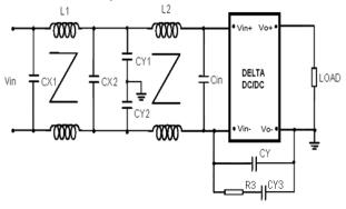
Figure 13-1: Recommended Input Filter
