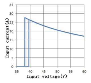
Figure 3: Full Load Input Characteristics
