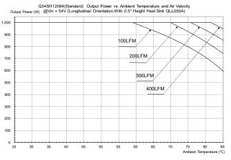
Figure 22: Output Power vs. Ambient Temperature and Air Velocity @Vin = 54V (Longitudinal Orientation, Airflow from Vout to Vin, With 0.5" Height Heat Sink QLL050A)
