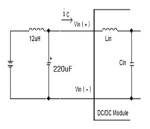
Figure 9: Test Setup Diagram for Input Ripple Current Note: Measured input reflected-ripple current with a simulated source Inductance of  $12\mu$ H. Measure current as shown above.
