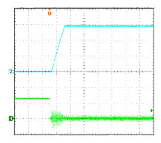
**Figure 5: Remote On/Off (negative logic) at full load** Vin=54V, I<sub>out</sub> = I<sub>o, max</sub> Time: 10ms/div. V<sub>out</sub> (top trace): 4V/div;
