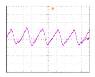
**Figure 10: Input Terminal Ripple Current**, ic, at max output current and nominal input voltage with  $12\mu$ H source impedance and  $220\mu$ F electrolytic capacitor (50 mA/div, 1us/div).
