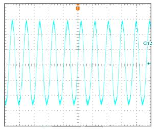
**Figure 12: Output Voltage Ripple and Noise** at nominal input voltage and max load current (10 mV/div, 1us/div) Load cap: 22uF\*5pcs ceramic cap, 330uF\*3pcs Oscon cap. Bandwidth: 20MHz.
