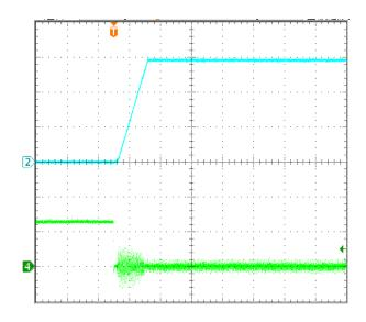
Figure 5: Remote On/Off (negative logic) at full load Vin=54V,  $I_{out} = I_{o, max}$ Time: 10ms/div.  $V_{out}$  (top trace): 4V/div;  $V_{remote On/Off signal}$  (bottom trace): 2V/div.
