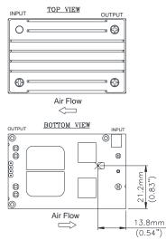
**Figure 21:** Hot spot 3 temperature measurement location The allowed maximum hot spot 3 temperature is defined at  $120 \C$ .
