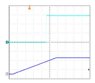
Figure 6: Input Voltage Start-up at full load
