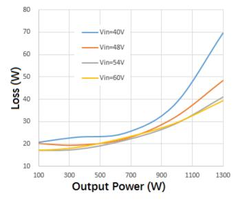
Figure 2: Loss vs. Output Power
