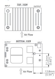
**Figure 19:** Hot spot 2 temperature measurement location The allowed maximum hot spot 2 temperature is defined at  $120 \,^\circ$ C.
