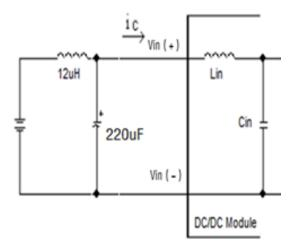
**Figure 9: Test Setup Diagram for Input Ripple Current** Note: Measured input reflected-ripple current with a simulated source Inductance of 12µH. Measure current as shown above.
