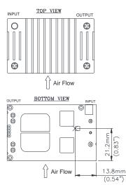
**Figure 17:** Hot spot 1 temperature measurement location The allowed maximum hot spot1 temperature is defined at 120 C.
