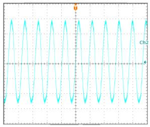
**Figure 12: Output Voltage Ripple and Noise** at nominal input voltage and max load current (10 mV/div, 1us/div) Load cap: 22uF\*5pcs ceramic cap,1000uF\*3pcs Oscon cap. Bandwidth: 20MHz.
