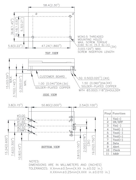
Pin 1~7 are copper alloy with matte tin plated over nickel under-plating. Pin 8~11 are copper alloy with gold flash plating.
