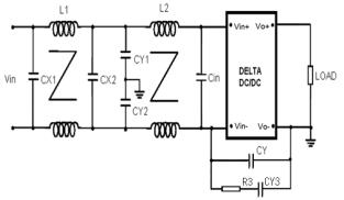
Figure 13-1: Recommended Input Filter
