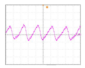
Figure 10: Input Terminal Ripple Current,  $i_c$ , at max output current and nominal input voltage with 12µH source impedance and 220µF electrolytic capacitor (50 mA/div, 1us/div).
