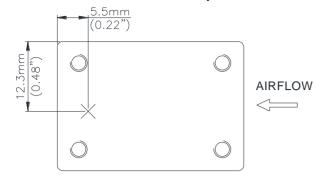
Figure 23: \* Hot spot 2 temperature measurement location. The allowed maximum hot spot temperature is defined at 110  ${\cal C}$
