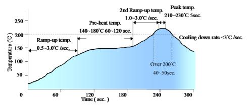
Note: The temperature refers to the pin of V48SC, measured on the pin +Vout joint.
