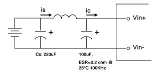
*Figure 9:* Test set-up diagram showing measurement points for Input Terminal Ripple Current and Input Reflected Ripple Current.
