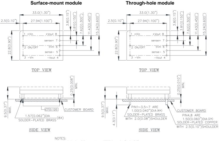
DIMENSIONS ARE IN MILLIMETERS AND (INCHES) TOLERANCES: X.Xmm±0.5mm(X.XX in.±0.02 in.) X.XXmm±0.25mm(X.XXX in.±0.010 in.)
