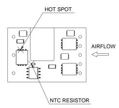
Figure 21: \* Hot spot 1& NTC resistor temperature measurement location. The allowed maximum hot spot temperature is defined at 120  ${\rm °C}$
