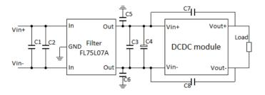
Figure 14 - EMI test schematic
