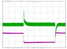
**Figure 8.2:** Output voltage response to step-change in load current 0A-3.2A-0A, max; di/dt = $2.5A/\mu$ s). Load cap: 10 $\mu$ F tantalum capacitor and 1 $\mu$ F ceramic capacitor. Top Trace: Vout (0.2V/div, 200us/div), Bottom Trace: lout (2A/div). Scope measurement should be made using a BNC cable (length shorter than 20 inches). Position the load between 51 mm to 76 mm (2 inches to 3 inches) from the module Note: for module V48SC12007NMFP
