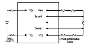
Figure 17: Effective circuit configuration for remote sense operation
