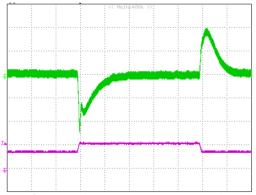
**Figure 8.1:** Output voltage response to step-change in load current (75%-50%-75% of lo, max; di/dt =  $0.1A/\mu$ s). Load cap: 10µF tantalum capacitor and 1µF ceramic capacitor. Top Trace: Vout (0.15V/div, 200us/div), Bottom Trace: lout (5A/div). Scope measurement should be made using a BNC cable (length shorter than 20 inches). Position the load between 51 mm to 76 mm (2 inches to 3 inches) from the module
