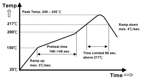
Note: The temperature refers to the pin of V48SC, measured on the pin +Vout joint.
