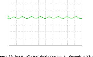
**Figure 11:** Input reflected ripple current,  $i_s$ , through a  $12\mu$ H source inductor at nominal input voltage and rated load current (20 mA/div, 2us/div)
